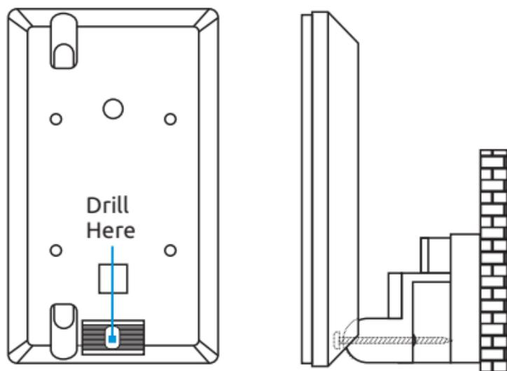
Drill a small hole through the back of the case in the location indicated, align the case back, then using the supplied screw attach the case back to pieces A and B.
