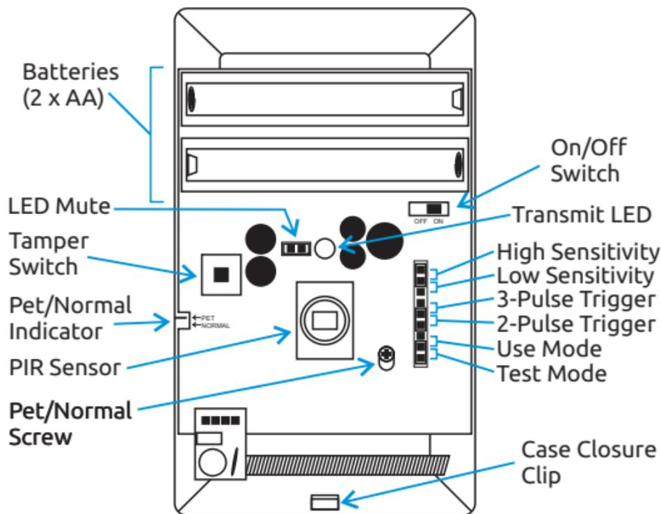
To change the battery or modify any of the jumper settings, depress the Case Closure Clip with a small screwdriver or similar object to open the case.
