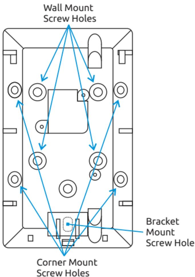
To install directly on a surface such as a wall, use the screw holes in the back of the case (note circuit board must be removed). There is a thin layer of plastic covering the holes, which can be easily pierced by a screw or nail.
