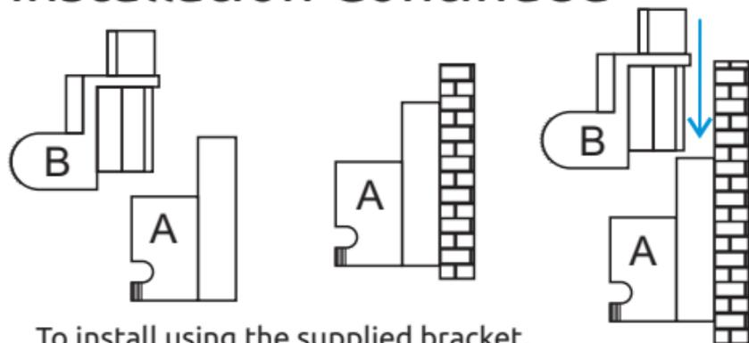
To install using the supplied bracket, attach piece A of the bracket to the wall (fasteners not included), then slide piece B downward into piece A.
